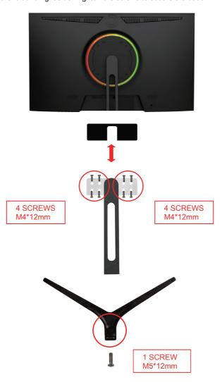
2. Install the hinge cover to the back of the neck.
