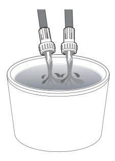
4 Connect the ends of the water supply hoses to the water supply intake connections at the top of the washer. Make sure that the rubber washers are in place. The water supply hose connected to the hot faucet must be connected to the hot water supply intake and the water hose connected to the cold faucet must be connected to the cold water supply intake.
