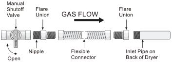
All connections must be wrench-tightened
