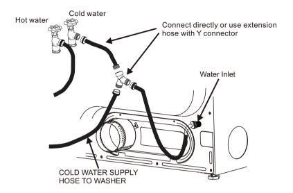
If possible install the "Y" connector directly, thread the short extension hose onto the COLD water supply and snug it by hand; then tighten it another ½ turn with pliers. Thread the "Y" connector to the short extension hose and snug it by hand; then tighten it another ½ turn with pliers.
