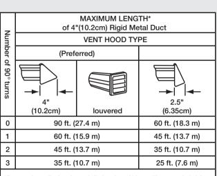
\*Do not install plastic or foil ducting. If installing semi-rigid ducting, do not exceed 8 ft (2.4 m) total duct length.
