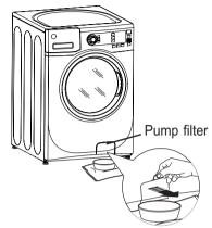
1. Using a coin or flat screwdriver in the notch on the door, open the access door.
