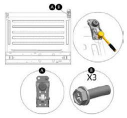
3. Unscrew and insert the hinge pin on the opposite side of the bottom hinge using an adjustable wrench and pliers.
