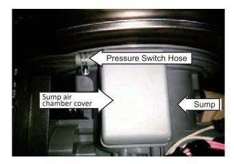
13. Remove the 2 clamps, sump outlet hose, and inlet hose from the sump.
