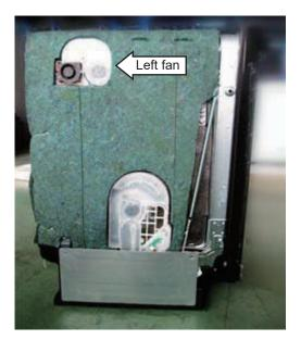
4. Open the door and rotate the fan nut and remove it from the left fan.
