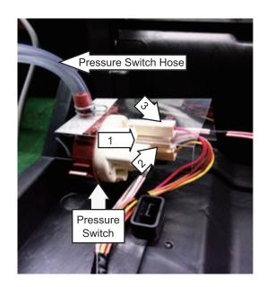
**Note:** When installing the pressure switch, ensure the switch is fully seated in the bottom of the base bracket.
