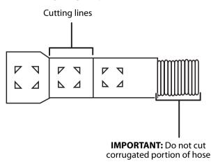
2 If a longer drain hose is required, you can add up to 42" (1.1 m) of length, for a total of 10 ft. (3.01 m) to the factory installed hose. Use 5/8" or 7/8" inside diameter hose and a coupler to connect the two hose ends. Secure the connection with screw-type hose clamps.
