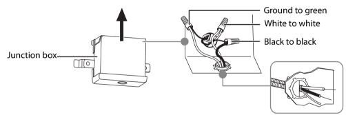
Insert wires through strain relief fitting and tighten
