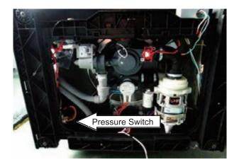
4. Release the snap joint that attaches the pressure switch to the base, and take out the pressure switch.
