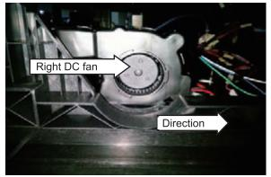
8. Release the snap joints and take the right DC fan motor out.
