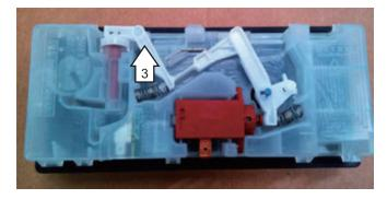
**Note:** Make sure the rubber seal is retained in the recessed groove before reinstalling the module to the door assembly.
