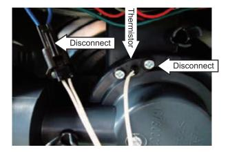
**Note:** Ensure the O-ring is retained in the thermistor before reassembly.
