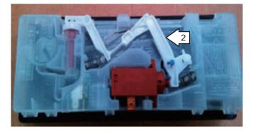
At the second activation, the lever lifts the connecting rod by the notch. This action lifts the rinse dispenser plunger (3) and releases the rinse agent. When deactivated, the lever returns to its original starting position.
