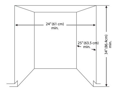
If installing into a corner, allow 2 in. (5.08 cm) min. clearance between dishwasher and adjacent cabinet, wall, or other appliances. Allow 25.63 in. (65.1 cm) min. clearance from the front of the dishwasher for opening the door.
