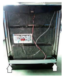
5. Remove the 2 Phillips-head screws from the Base side panel on each side.
