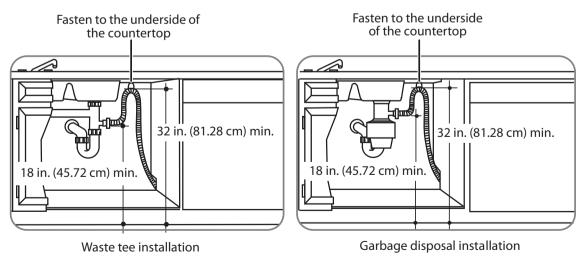
4 If connecting the drain line to a garbage disposal, make sure that the drain plug has been removed. Your dishwasher will not drain if the plug is left in place.
