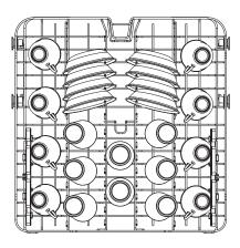
8 place settings standard loading pattern (For best washing performance, the upper rack should be in the raised position.)
