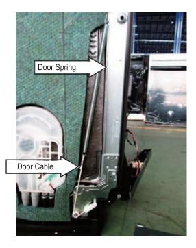
7. Open the inner door at 10°, and lift the door until the door hinge seperate from the type D pin.
