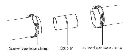
3 Secure the drain hose to the air gap, waste tee, or garbage disposal with a screw-type clamp, using the appropriate method below. See "Drain preparation on page 6" on page 6, if you do not know which method to use.
