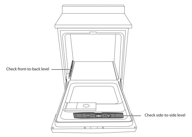
2 Level the dishwasher by adjusting the four leveling legs individually.
