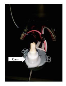
7. Disconnect the 2 wires from the micro s/w.
