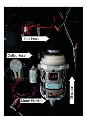
**Note:** Factory-installed hose clamps are not reusable. When installing a water inlet valve, drain pump assembly, motor pump assembly, or sump assembly, replace the old clamps with new screwtype hose clamps provided. The screw-type hose clamps are available separately.
