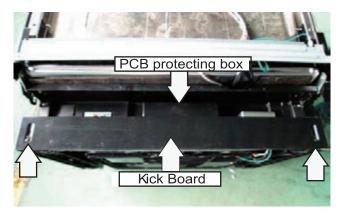
5. Remove 2 Phillips-head screws on the PCB protecting box.
