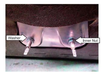
11. Lift the back side of the element and release it from the 2 retainers.
