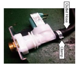
**Caution:** The clamp is easily damaged during removal and should not be reused. Use the screw-type hose clamp provided with the new valve.
