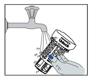
Because hard water chemicals will clog the spray arm jets and bearings, it is necessary to clean the spray arms regularly. Wash the arms in soapy, warm water and use a soft brush to clean the jets. Replace them after rinsing thoroughly.
