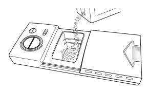
3. After pouring the detergent into the compartment, close the lid, first pushing (1) and then pressing on it (2) until you hear the click.
