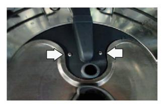
2. Release the snap joints shown in the figure. Then take out the nozzle duct and lower spray seat.
