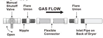
All connections must be wrench-tightened
