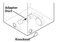
3. Preassemble a 4 inch (10.2cm) elbow to the next 4 inch (10.2cm) duct section, and secure all joints with aluminum tape. Be sure that the male end of the elbow faces AWAY from the dryer.
