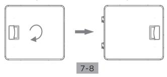
9 Align the hinges on the door with the hinge screw holes on the front of your dryer, then secure the door with the four screws you previously
