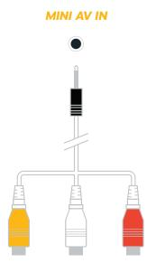
Connect a USB device for browsing photos, music, or videos. Connect a composite video cable and left-right audio cables from an external AV device (AV adapter included). Connect a composite video cable and left-right audio cables from an external AV device.
