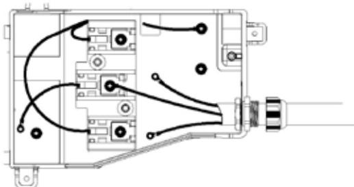
5. Connect the neutral ground conductor under the screw B. Then connect the remaining supply cord wires under the outer terminals of the block. Tighten all screws. After every connection is completed, tighten strain relief clamp in order to secure the supply cord. Finally, cover up the box cover.
