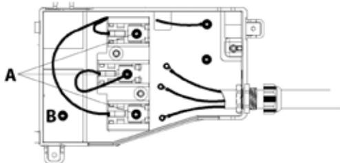
4. Remove the neutral ground conductor from central terminal and connect the neutral wire of the supply cord under the central terminal of the block. Tighten the screw.
