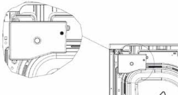
2. Remove the clamp of the strain relief which has already attached on your machine. Then pass the clamp through the supply cord and put the supply cord through the main body of the strain relief. Be sure that wire insulation of the cord inside the strain relief.
